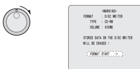
6 Turn the jog dial to select "FORMAT START", and then turn the shuttle dial clockwise.
